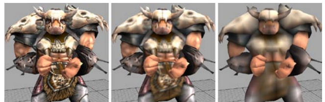
TGE Orc with various mip map levels: mip map #0 512x512 (far left), mip map #2 128x128, mip map #4 32x32. A seam down the middle of the object becomes more apparent as the texture is scaled smaller for the various mip maps.
